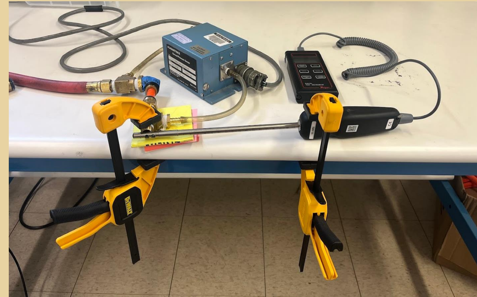
An example of the testing setup, configured for a fitting test.
